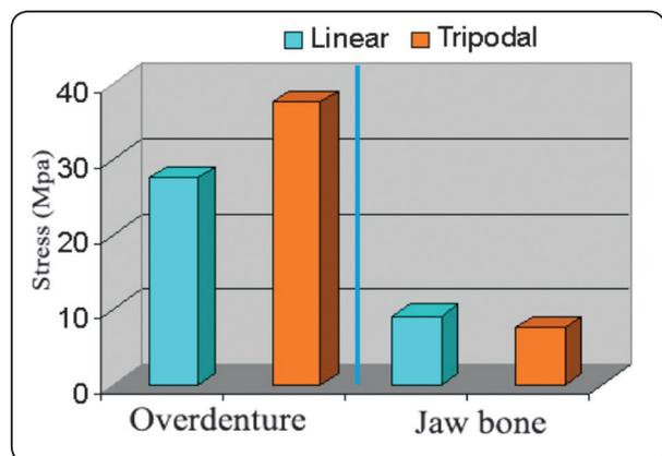
Fig. (8) maximum recorded stresses around the denture and jaw bone in linear or tripodal implant arrangement
