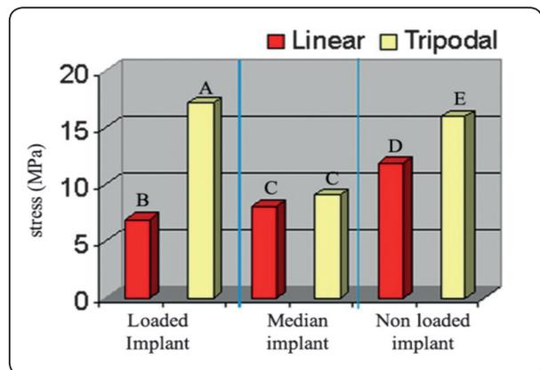
Fig. (7) maximum recorded stresses around the implants in linear or tripodal (staggered) situation for mandibular overdentures
