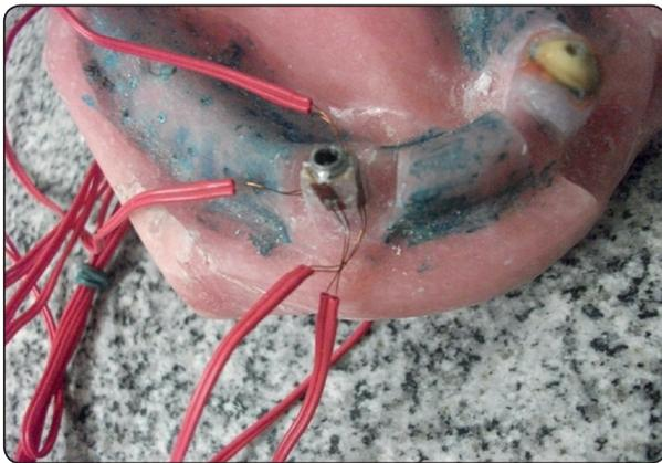
Fig. (4) The simulated model with strain gauges attached around the implant
