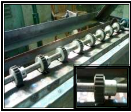
Fig. (6) : Developed seeder feeding shaft and its reels
