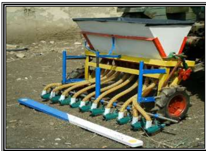
Figure (2):The developed seed drill
