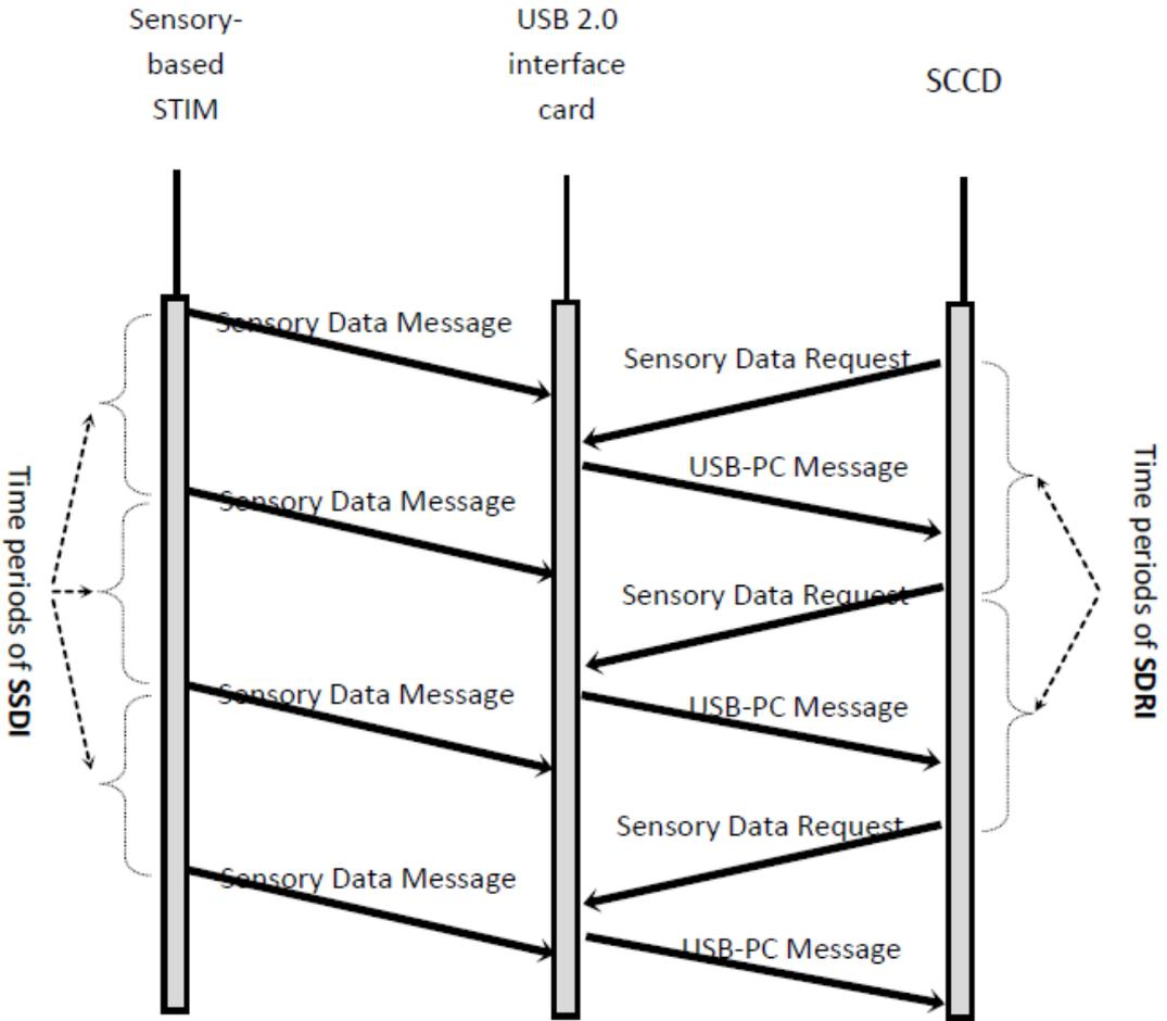
Fig.14 Communication scenario between SCCD and sensor-based STIM
