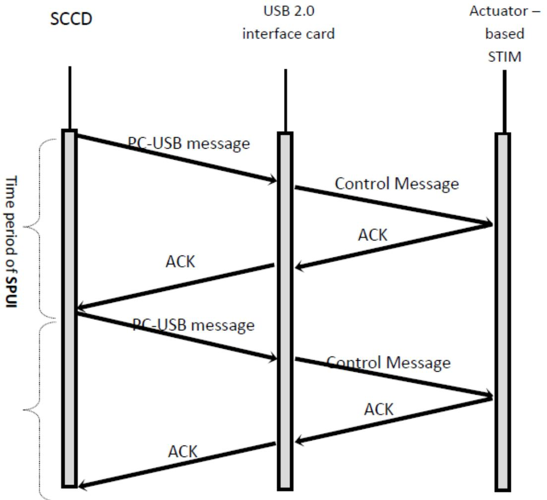
Fig.15 Communication scenario between SCCD and actuator-based STIM
