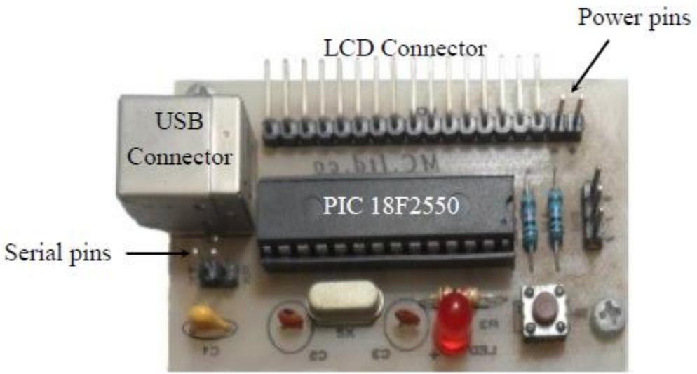
Fig.7 Practical circuit of USB 2.0 interface Card
