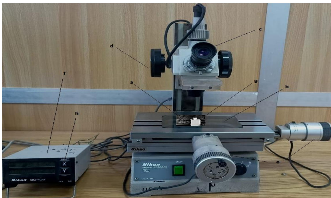
Figure. 1 The Nikon-10 Measurescope (Nikon Measurescope UM-2, Nikon, Tokyo, Japan) components showed (a) the specimen, (b) the observation table, (c) the eyepiece, (d) Major adjustment, (e) Two digital fine adjustment tool, (f) Digital readout unit, (g) right angles metal stand, (h)reset button.
