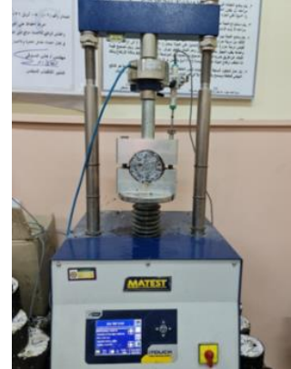
Figure (8): Marshall test Device
