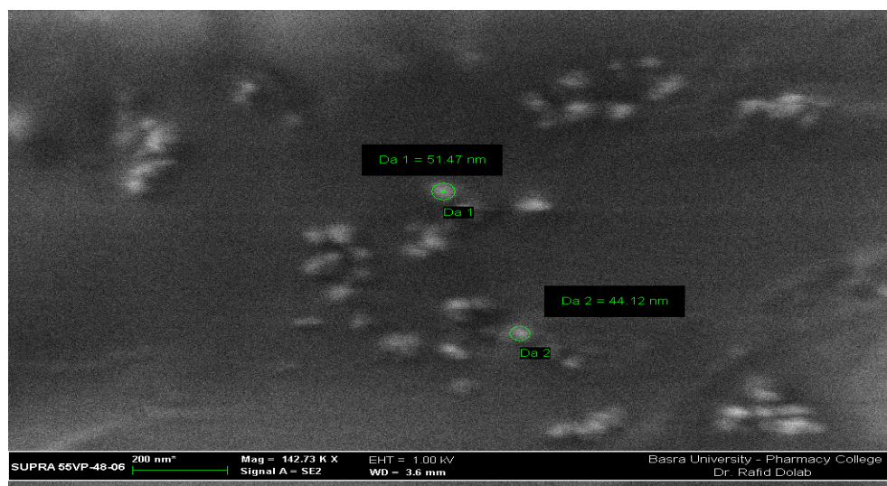
Fig. 9. SEM micrograph of (Cs-Arg) nanoparticles.
