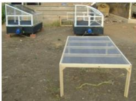
Fig. 3. Wooden frame of natural sun drying beside the two solar dryers
