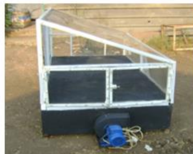
Fig. 1. Schematic diagram and the plate of lean-to solar dryer
