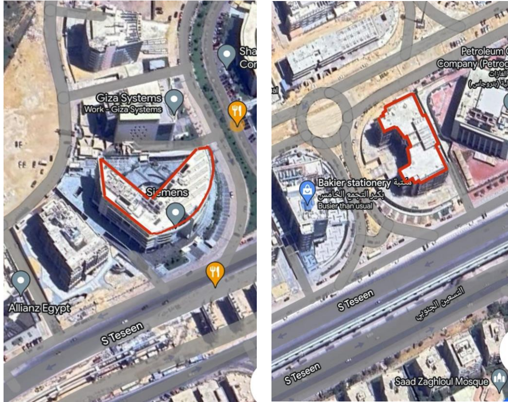
Fig(2c): Effect of curved buildings , the building's major axis perpendicular to the direction of the highway and its site is relatively far from traffic way and semi enclosed courtyard on noise mitigation (case study ) (Researcher)
