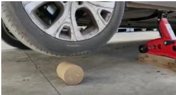
Figure 15 Non formal test, developed with a car and the sample for an exhibition. The specimen was not broken after applying all the load.
