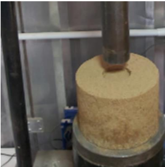
Figure 12 CBR specimen removed from the mould and placed again to show the impressive results. The specimen has a 30% of OMC replacement with SS21.
