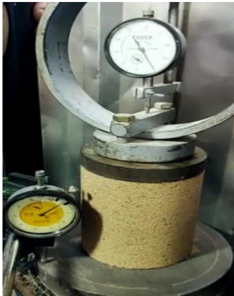
Figure 9 Specimen with 20% solution of SS21, during test.
