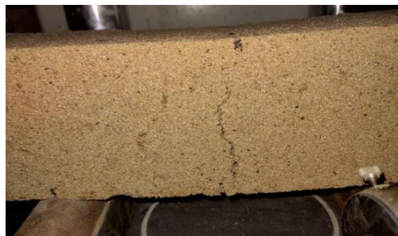
Figure 17 Beam on failure during test. 30% of SS21.
