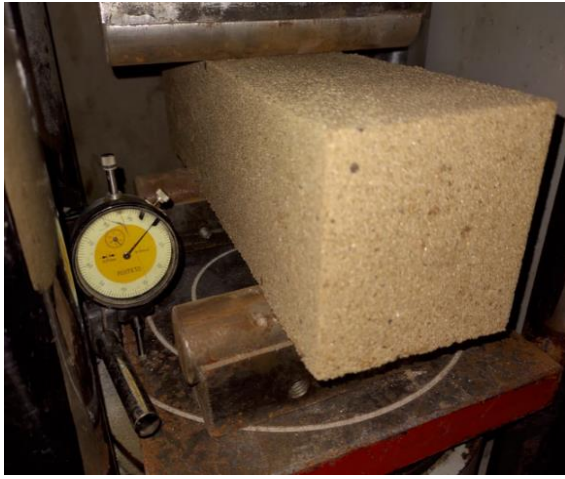
Figure 19 Beam during test. 30% of SS21.
