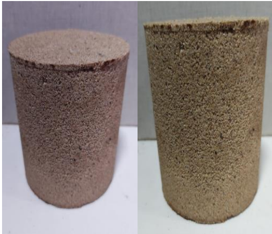
Figures 8a and 8b Specimen with 20% solution of SS21, before being tested.
