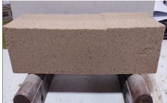
Figure 16 100x100x350mm beam of sand with 30% of SS21.
