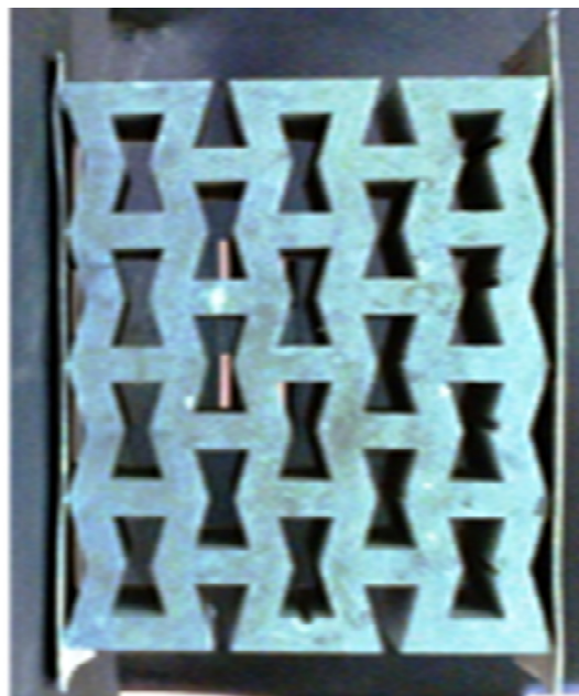
Figure (3). HSP fabricated by using wire-cutting machines.
