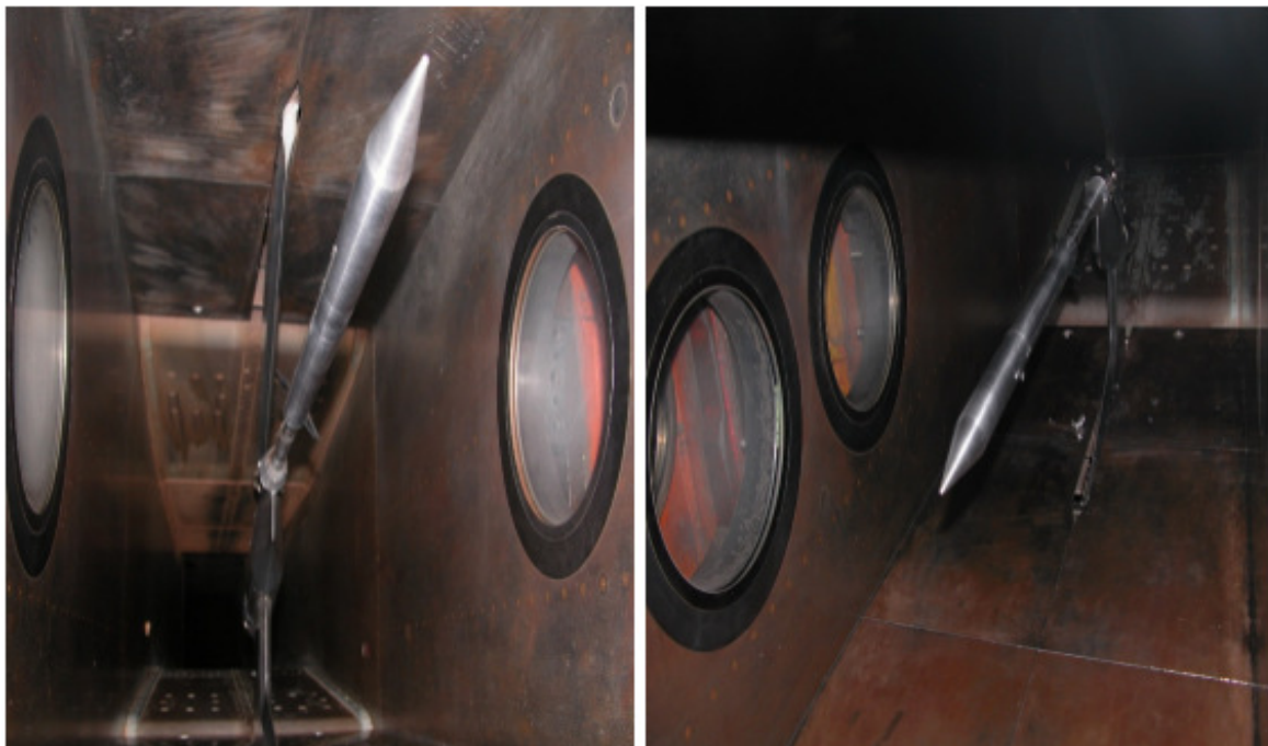
Figure 2. Model installation in the wind tunnel test section.
