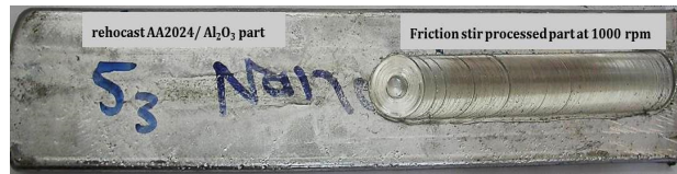
Fig.1. Example of semi-solid processed AA2024/Al 2 O 3 nanocomposite plate.
