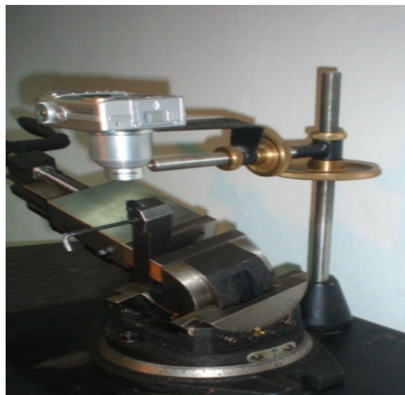
Fig.3. CCD camera equipped with changeable standard lenses and adapter, 2D stand and 3way vice.
