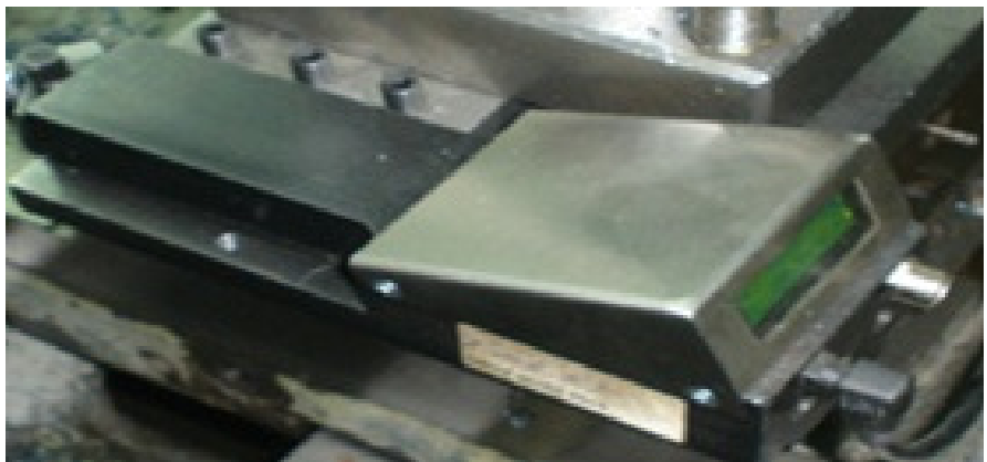
Fig.5. Force dynamometer, the tool holder and the LCD display.
