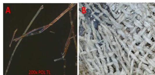
Figure 6: Investigation of the textile: (A) Textile is identified as linen. (B) Textile quality 16x24 threads per 1cm 2
