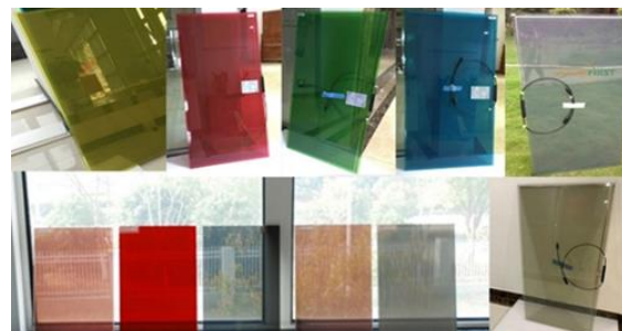
Fig.6. Examples of transparent Amorphous thin-film panels
