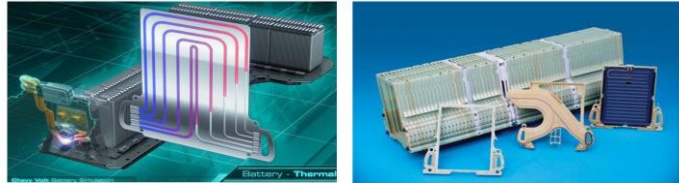
Fig .21 Liquid cooling systems demonstrated by Chevy Volt [50]
