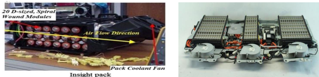
Fig. 9. Air cooling systems demonstrated by Honda Insight [8] and Toyota's Highlander [29]
