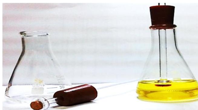
**Fig. 1:** Cells used for the in-vitro release test from tablets.
