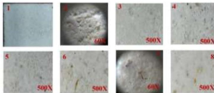
Fig. 8: shows the results of group (F) after applying the nanocomposite, after wet-drying cycles, and after weathering cycles with sodium chloride salt.
