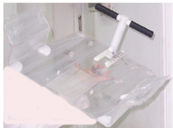
Fig. 5: Wing board used a method for patients positioning reproducibility.
