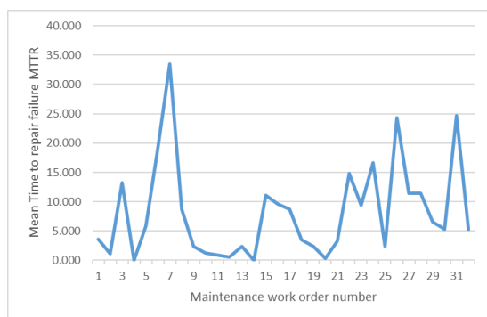
Figure 5: Mean Time to Repair Failures for the Rolling Machine.
