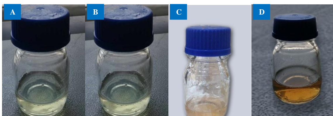
Fig. 6. Mixture of aqueous tomato extract and silver nitrate (1mM) A,C (1:1, 10 ml \text{AgNO}_3 + 10 ml tomato extract) before and after reaction and B,D (1: 2, 10 ml \text{AgNO}_3 + 20 ml tomato extract) before and after reaction.
