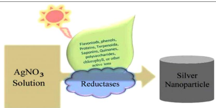
Fig.1. Mechanism of AgNP Phytosynthesis by using concepts of metal reduction, AgNP phytosynthesis and reduction by reductases (20).
