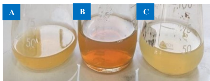
Fig. 4. Reaction tubes after 2 hrs. of reaction containing aqueous tomato extract and AgNO 3 solutions at different dilutions :
