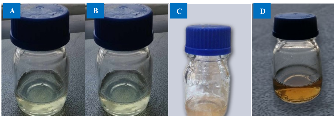
Fig. 6. Mixture of aqueous tomato extract and silver nitrate (1mM) A,C (1:1, 10 ml AgNO 3 + 10 ml tomato extract) before and after reaction and B,D (1: 2, 10 ml AgNO 3 + 20 ml tomato extract) before and after reaction.
