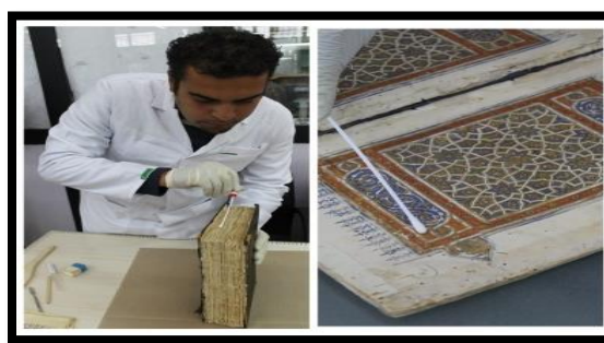
Fig.1. Swabs from the edges (139B) and the pigments (139m I, 139II, 139III, 139IV, 139V).
