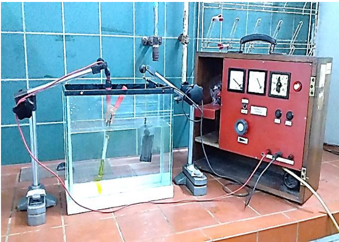
Figure 4: Pyrex glass cell (hydrogen pre-loaded specimen in solution aqueous 0.1N H 2 SO 4 , /100mA/Cm 2 /pH=1.32)/ [13], [14], [21], [23], [26], [28], [30], [31].
