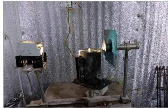
Figure 4- Plastic shrinkage settlement device
