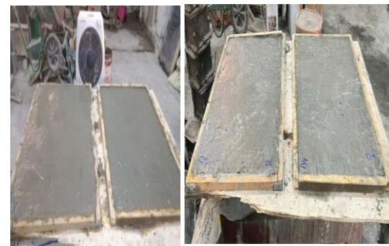
Figure 6- Plastic shrinkage panel tests
