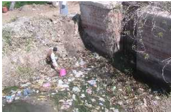
Figure (9) Collecting sample for the point of inlet ( Just before the existing screen).
