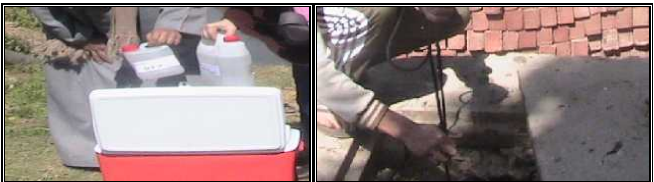
Figure 3 (a) The Preservation of the collected samples (b) Collection of a sample from a manhole.
