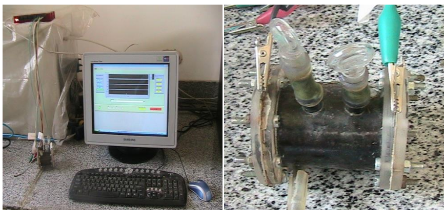
Figure 1: membrane less air cathode single chamber microbial fuel cell composed of anode and cathode electrodes connected with wire to close the circuit.
