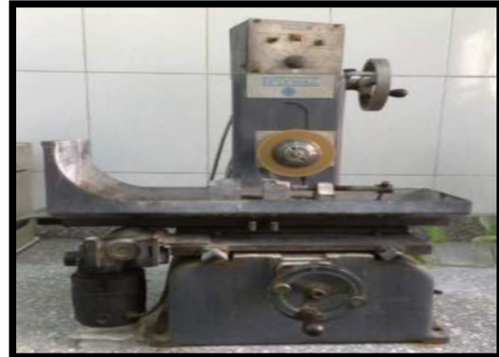
Figure 6. A photograph showing the cutting machine used for sectioning the teeth specimens.
