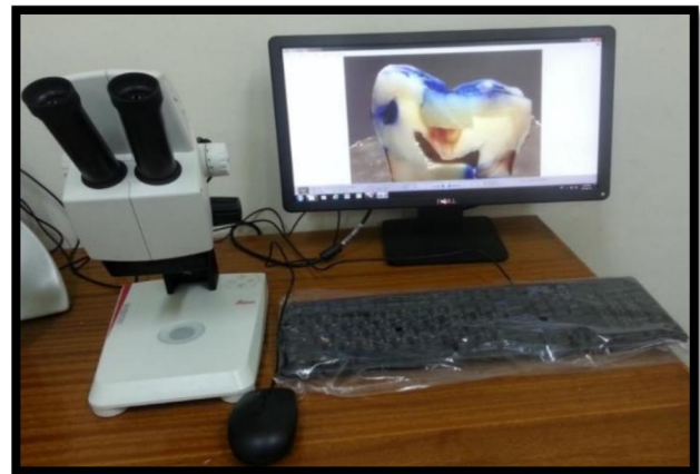
Figure 7. A photograph showing the stereomicroscope used for examining the marginal leakage.
