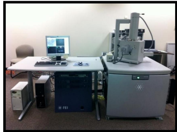
Figure 10. A photograph showing SEM used for evaluation of marginal gap.
