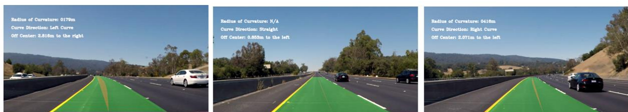
Fig. 6. Curvature estimation and directional analysis
