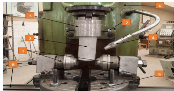
Fig.3 The Experimental setup of nosing process.
