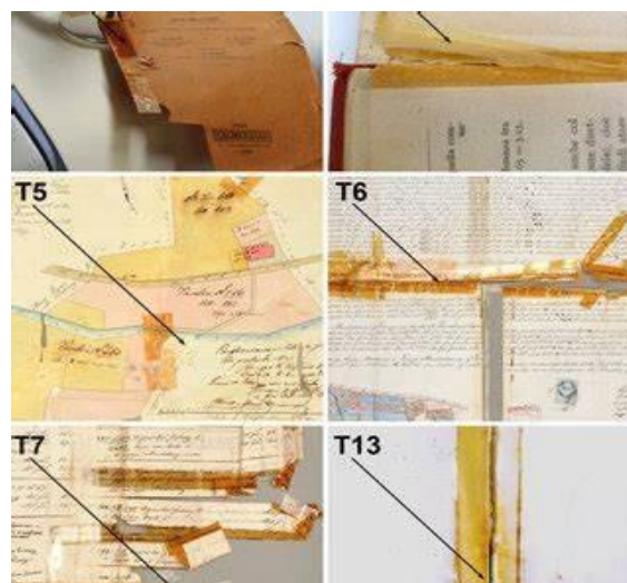
Figure 2. Dark brown staining along the split spine fold of paper caused by pressure-sensitive adhesive tape (PSAT) on some of the maps and book papers [9].
