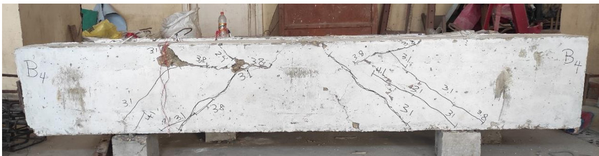
Fig. 8. Crack patterns at failure of specimen (B3)
