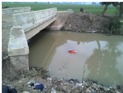
Figure 1: Velocities and bathymetry measurements at the six cross sections using ADCP device.
