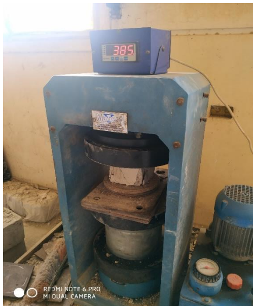
Fig. 3. Compression test machine used for donating the compressive strength on 100 mm cubes for each mix at 28, 56 and 92 days.
