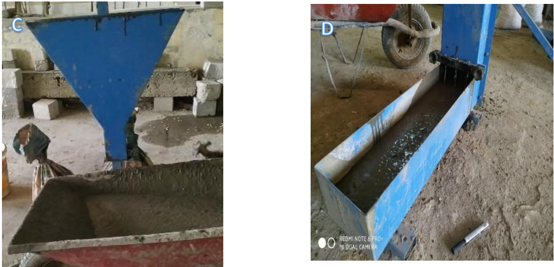
Fig. 2. Testing SCC at fresh state for examining the flowability, viscosity and passing ability according to EFNARC: (A) slump flow test; (B) j-ring test; (C) v-funnel test and (D) l-box test.
