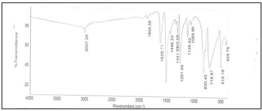
Fig (1): FTIR spectrum of compound AH1.
