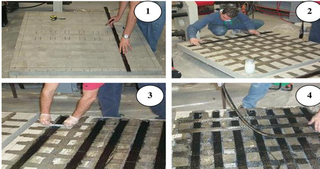
Fig. 1: Marking; (2) impregnating and bonding the carbon strips to the concrete slab; (3) rolling away extra glue; (4) adding more layers. [12]
