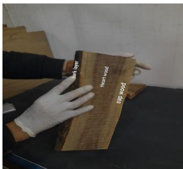
Fig.1, Shows the three parts of wood (heart wood - sap wood - park layer)
