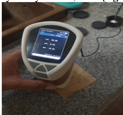
[figure 12]: The equipment used to measure the color change of experimental samples
