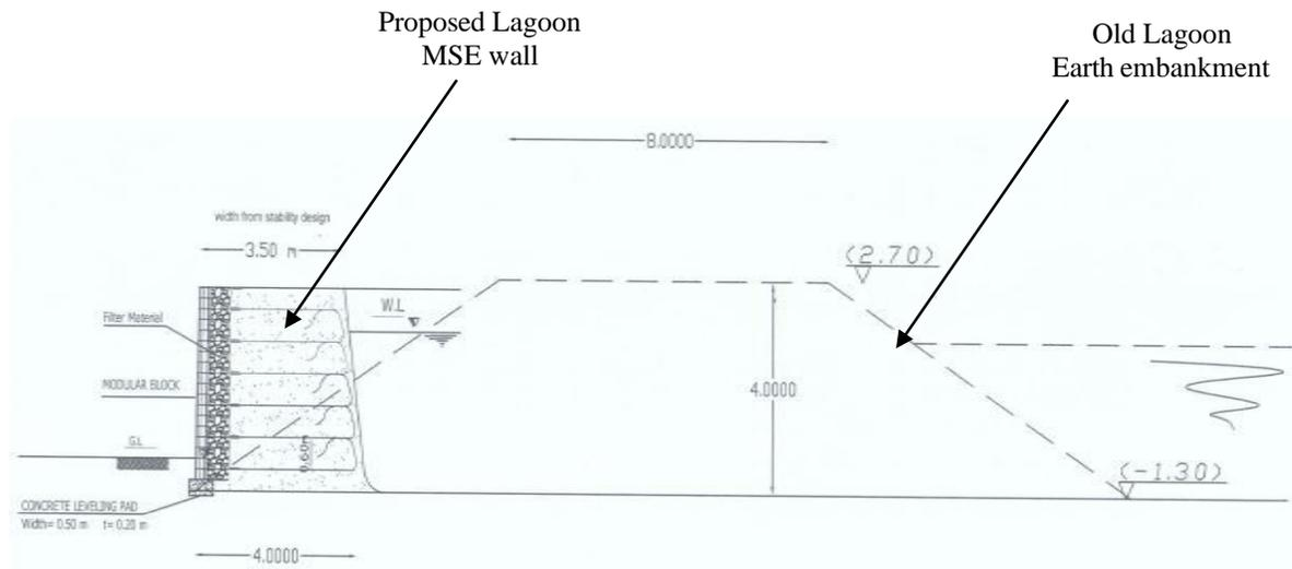
Figure (11) Section shows comparison between the geometry of the proposed MSEW and traditional embankment existing earth wall
