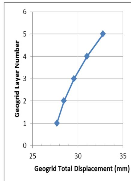
Figure (11) Induced lateral displacement in geogrid layers
