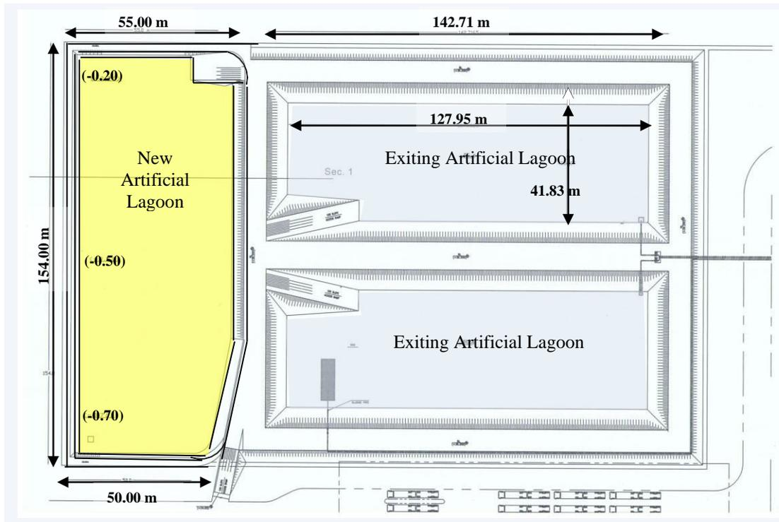
Figure (3) Plan of the position of the new required artificial lagoon close to the existing lagoons
