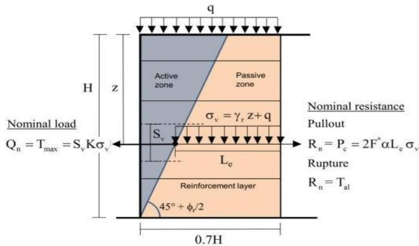
Figure (5) Problem geometry, internal pull-out and geogrid mechanically stabilized earth (MSE) wall rupture limit states
