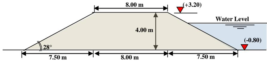
Figure (2) Cross-section (1-1) in the earth side of the existing lagoons
