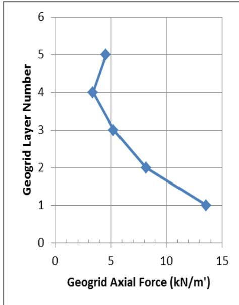
Figure (9) Profile of Axial Force in wall geogrid layers
