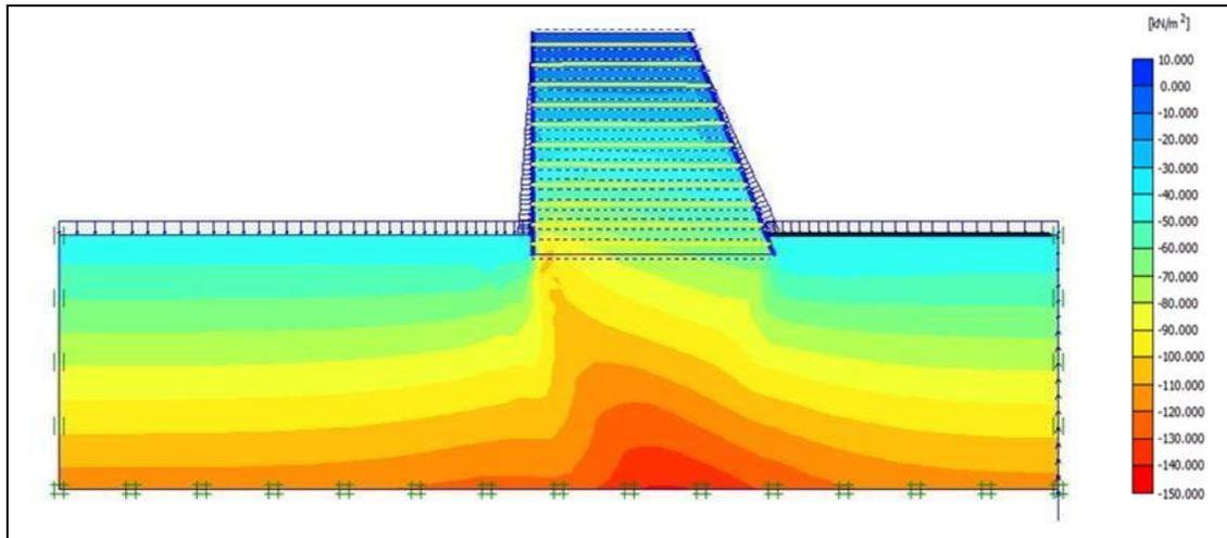
Figure (8) Distribution of mean stress in the MSE body and the foundation soil
