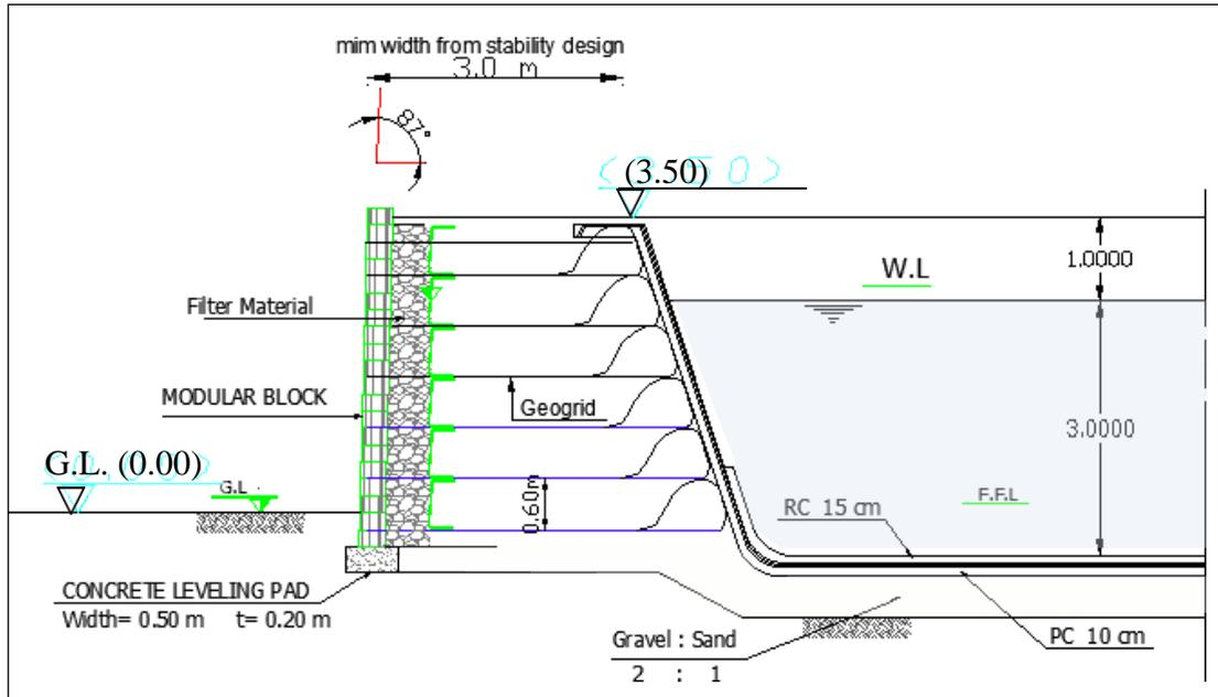
Figure (6) Geometry of the proposed MSE wall for the new artificial lagoon
