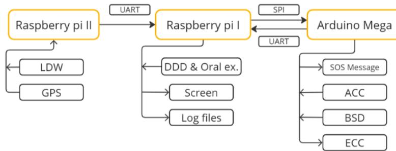
Figure 18 integration's block diagram
