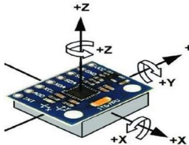
Figure 11 the rotation motion of Gyroscope in (x, y, z) axis
