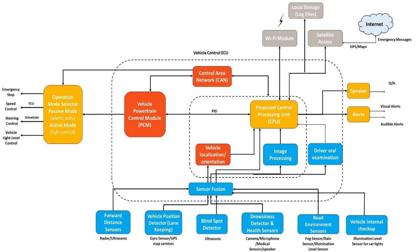
Figure 2 IDAS block diagram
