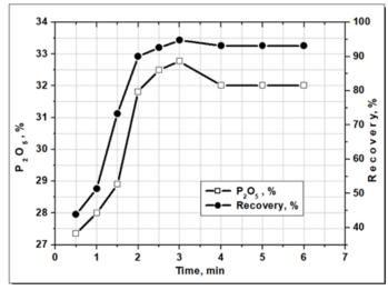
Fig (10): Effect of flotation time on the content; % and recovery % of apatite (100-75 µm particle size, 1.5 g/kg sesame oil collector, 6g/kg corn starch depressor, pH pulp 10 and 1:3 S/L ratio, 2000 RPM and 1.6 cm/s air superficial velocity) at 25°C.
