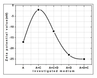
Fig (4): Zeta potential of apatite before and after mixing with collector and depressor at pH9 *A is apatite, C is Collector and D is depressor*
