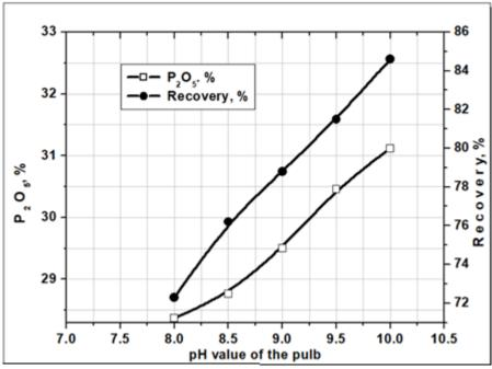
Fig (7): Effect of pH of the pulp on the content % and recovery % of apatite (100-75 μm particle size, 1.5 g/kg sesame oil collector, 6g /kg corn starch depressor and 1:3 S/L ratio, 2 min flotation time, 2 cm/s air superficial velocity, 2000 RPM) at 25 °C.
