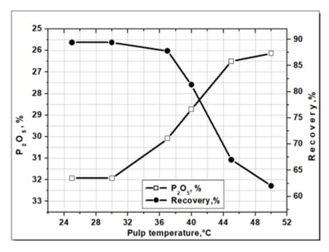
Fig. (9): Effect of the pulp temperature on the content; % and recovery % of apatite (100-75 µm particle size, 1.5 g/kg sesame oil collector, 6g/kg corn starch depressor, pH pulp 10 and 1:3 S/L ratio, 2 min flotation time, 2000 RPM) with 1.6 cm/s air superficial velocity.
