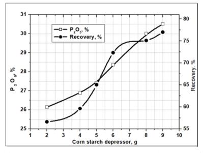
Fig. (6): Effect of gelatinized corn starch as a depressor /g on the content; % and recovery; % of apatite (100-75 μm particle size, 1.5 g/kg sesame oil soap collector, 1:3 S/L ratio, pulp pH 8, 2 minutes flotation time, air superficial velocity 2.0 cm/s, 2000 RPM) at 25 °C.
