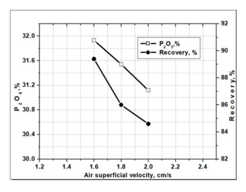
Fig (8): Effect of air superficial velocity on the content; % and recovery % of apatite (100-75 μm particle size, 1.5 g/kg sesame oil collector, 6g/kg corn starch depressor, pH pulp 10 and 1:3 S/L ratio, 2 min flotation time, 2000 RPM) at 25 °C.
