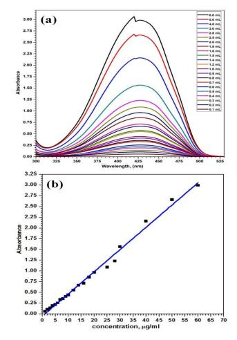
Fig (7): The absorption spectra of tartrazine with various concentrations (0.1 - 6 mL) and application of Beer's law for tartrazine using optimum conditions.
