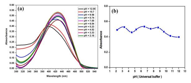
Fig (2): Absorption spectra of tartrazine at  $\lambda_{max}$ = 427 nm (a) and the absorption value of tartrazine (b) using a universal buffer with different pH [pH=2-12].
