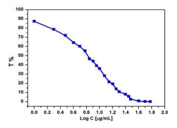
Fig (8): Ringbom plot for tartrazine by using optimum conditions.
