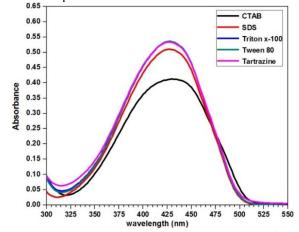
Fig (4): Absorption spectra of tartrazine without surfactant and by using different surfactants.
