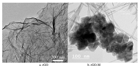
Fig. (4): TEM images of (a.) rGO; and (b.) rGO-M.
