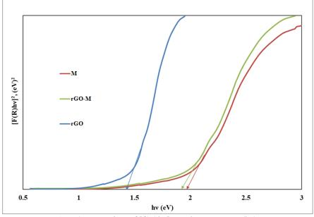
Fig. (7): Tauc plots of  $[f(R)hv]^n$  vs photon energy (hv).
