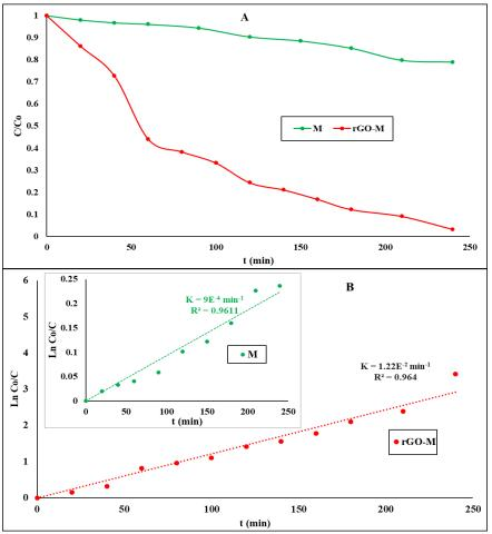
Fig. (8): A. Photocatalytic degradation of the MB dye by M and rGO-M photocatalysts under visible light irradiation: reaction conditions: (lamp power 160 W, filter  $\lambda$ = 420 nm, catalyst weight 1 gL<sup>-1</sup>, dye conc. 10 ppm). B. The kinetic fits for the same reactions.
