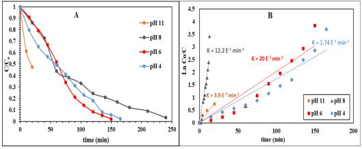
Fig. (8): A. Effect of change Fig. (9): Effect of pH on the degradation activity of the rGO-M photocatalyst towards MB under Vis. light illumination, reaction conditions: (lamp power= 160 W, filter  $\lambda$ =420 nm, catalyst load 0.5 g/L, 1.0 g/L and 2.0 g/L dye conc. 10 ppm). B. The kinetic fits for the same reactions.
