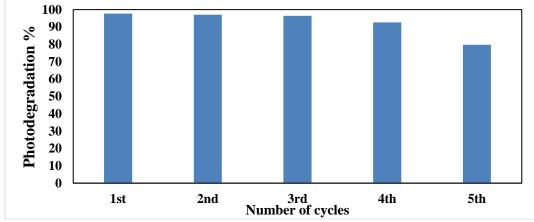
Fig. (13): Recycle test during degradation of MB using rGO-M as a photocatalyst under Vis. illumination.
