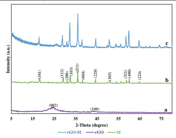
Fig. (1): XRD patterns of rGO, (a); Mn<sub>3</sub>O<sub>4</sub>, (b) and rGO-M (c).
