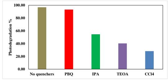
Fig. (12): Effect of reactive scavengers on the degradation activity of the rGO-M nanocomposite towards MB under Visible light and reaction conditions: (lamp power= 160 W, filter  $\lambda$ =420 nm, catalyst load 1.0 g/L, dye conc. 10 ppm).
