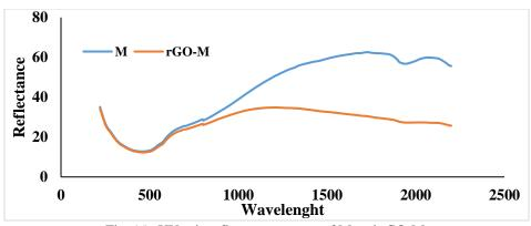
Fig. (6): UV-vis reflectance spectra of M and rGO-M.
