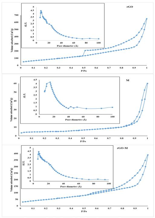
Fig. (3): N2 adsorption-desorption isotherms of rGO, M and rGO-M.
