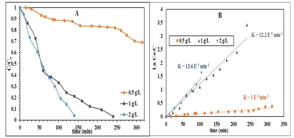
Fig. (10): (A) Effect of catalyst weight on the degradation activity of the rGO-M photocatalyst towards MB under Vis. light illumination: reaction conditions: (lamp power= 160 W, filter  $\lambda$ =420 nm, catalyst load 0.5 g/L, 1.0 g/L and 2.0 g/L dye conc. 10 ppm); (B) The kinetic fits for the same reactions.
