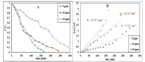
Fig. (11): (A)The degradation activity of the rGO-M photocatalyst towards MB with different concentrations under Vis. light illumination: reaction conditions: (lamp power= 160 W, filter  $\lambda$ =420 nm, catalyst load 1.0 g/L, dye conc. 10 ppm); (B). The kinetic fits for the same reactions.
