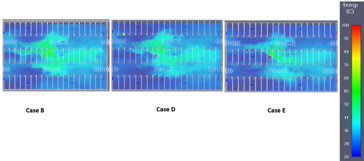
**Figure.10:** Temperature contours for cases B and D-E
