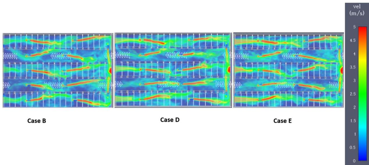
**Figure.11:** Velocity contours stagnation points for cases B and D-E
