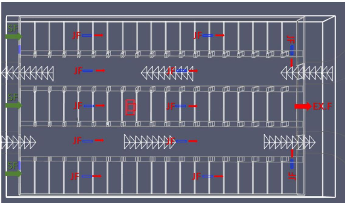
**Figure.3:** Second approach with three supply fans
