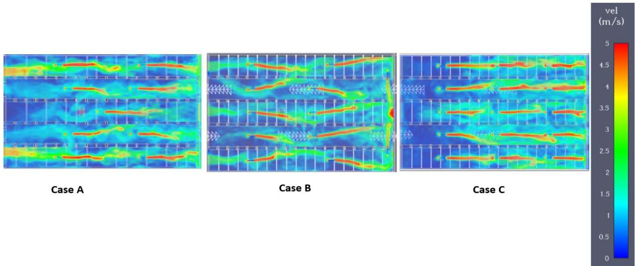
Figure.8: Velocity contours and stagnation points for cases A-C
