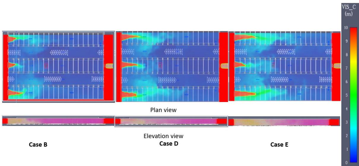
Figure.9: Visibility contours for cases B and D-E
