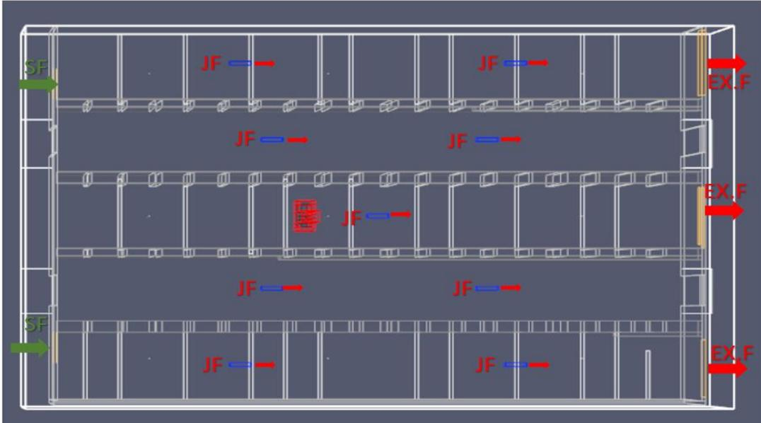
**Figure.2:** First approach with two supply fans
