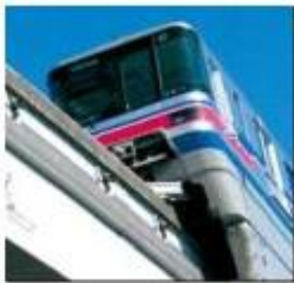
Fig. 1. Straddle-type Monorail System
