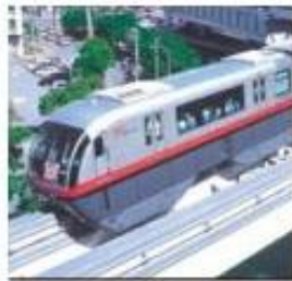
Fig. 1. Straddle-type Monorail System
