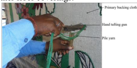
Figure 2. Tufting of Pile Yarn on Primary Backing Fabric [6]
