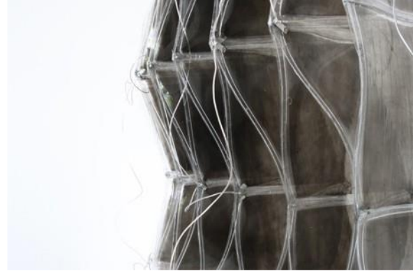
Figure 9: ShapeShift | EAP with carbon based electrodes for façade applications | Image by Manuel Kretzer
