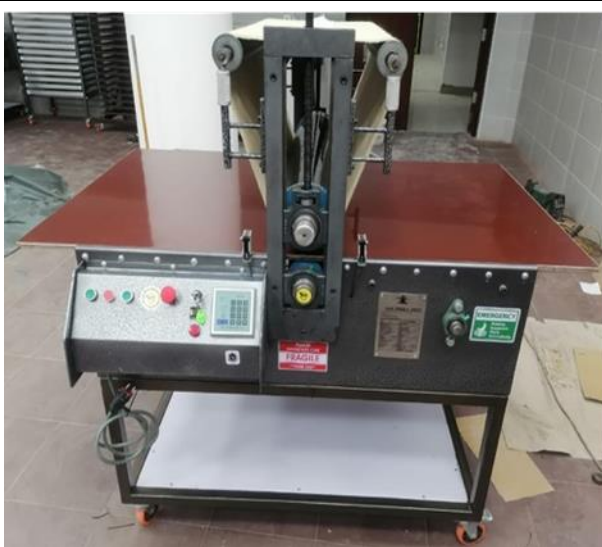
Fig. 14: Relief printmaking horizontal presses and attempts to fill the spaces around the printing block Source: Invented by the researcher: electric intaglio printmaking press that designed and made by the researcher inside the Egyptian – Russian university and the method of wooden screen.
