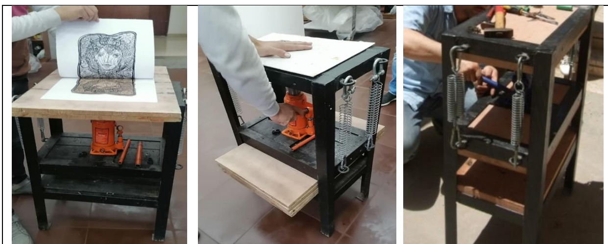
Fig. 29: A panoramic image for relief printmaking machine that invented and executed by the researcher using hydraulic 1.5 tons capacity crane that measures 40 cm width × 60 cm length × 85 cm height. Source: (The researcher: The printmaking labs of Alexandrian university and Egyptian Russian University)
