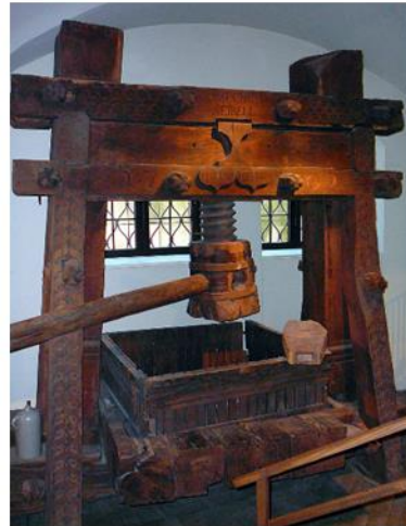
Fig .3: Early modern wine press screw presses , which inspired Gutenberg to design the moveable characters press with screw press
