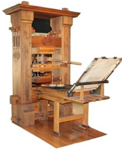
Fig .4: wooden screw printing press, invented in 1450 by Johannes Gutenberg (1398 – 1468)
