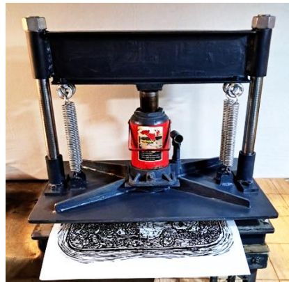
Fig. 35: Relief printmaking machine of high-pressure hydraulic cranes at capacity of 20 tons, invented by the researcher:
