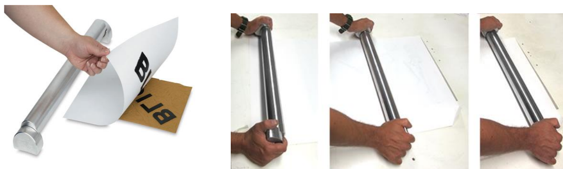
Fig. 16: Portable and rolling pressure cylinders for relief printmaking
