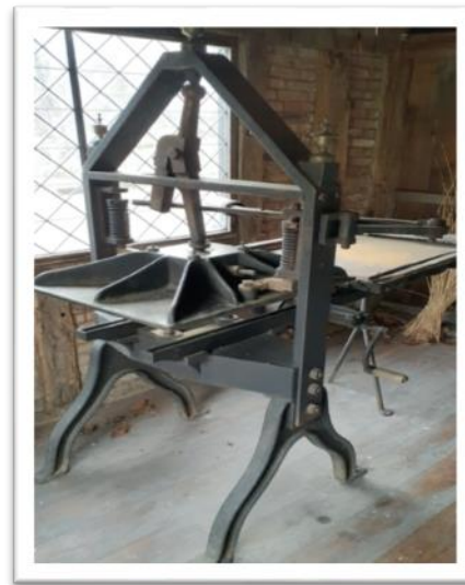
Fig .5: Ramage screw Press 1750, Scottish (1772-1850 Adam Ramage) . 1820 after inventing the vertical metal pressure bar method to ensure the height of metal printing cylinder easily after completing the pressure https://letterpresscommons.com/press/ramage-screw-press/
