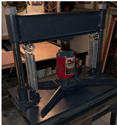
Fig. 35: Relief printmaking machine of high-pressure hydraulic cranes at capacity of 20 tons, invented by the researcher:
