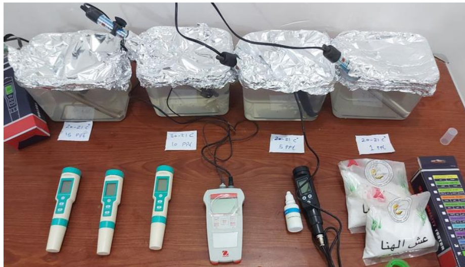
Fig. 2. Designing an oxygen consumption experiment in plastic tanks with measuring devices and thermometers installed to adjust the temperature
