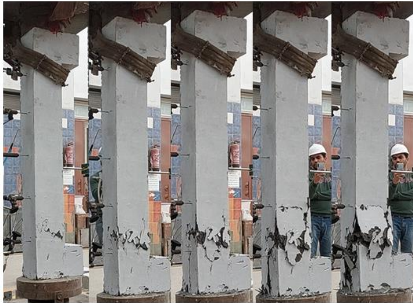
Fig 5: Shear Failure Pattern of Column 6Cs15.
