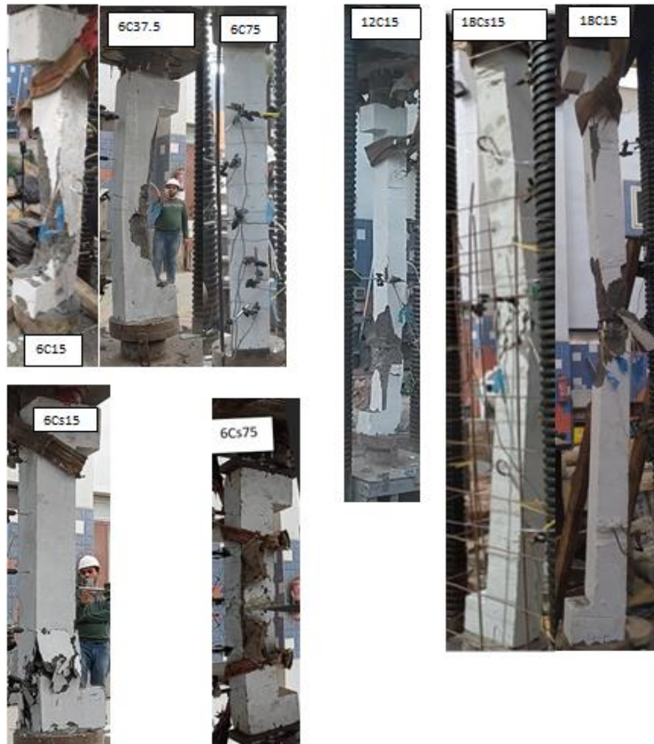
Fig 4: Columns Failure Pattern.
